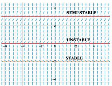
The stability of equillibrium solutions can also be found by evaluating the second derivative at the critical y-values. If d/dy(dy/dx) ( $y_c$ ) < 0, then a stable solution exists.
